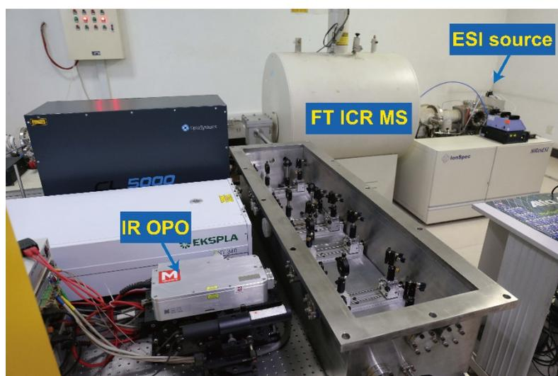
**Figure 2.** The experimental setup for IRMPD experiments in Nankai University, based on a 7 T FT ICR mass spectrometer (Ionspec) and a tunable optical parametric oscillator (OPO) laser (Msquares).
