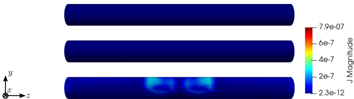
Fig. 18 Simulation results for RVE 1 for the electric current density \mathbf{J} [A/m 2 ] with \kappa_1 = 1 \cdot 10^2 S/m (top), \kappa_1 = 1 \cdot 10^4 S/m (in the middle) and \kappa_1 = 1 \cdot 10^6 S/m (bottom), t = 50
