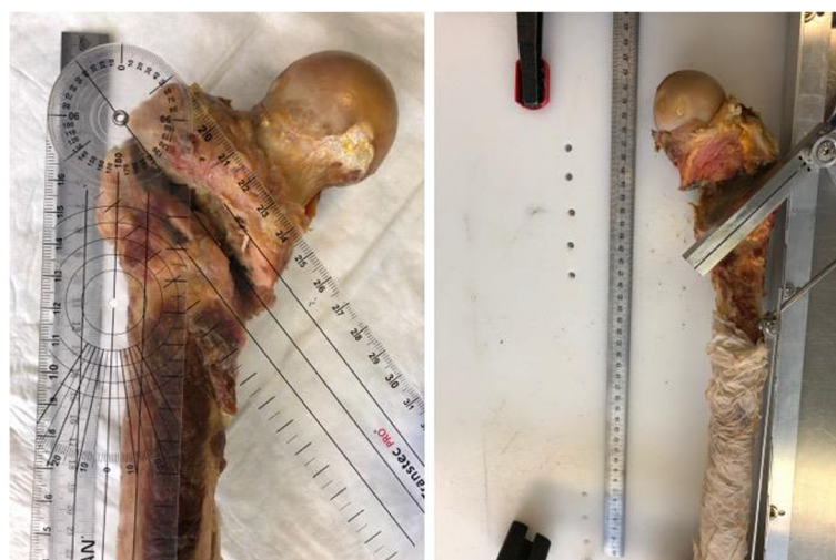
Fig. 4 Exemplified images of a fractured (left) and an osteotomized (right) specimen; on the left, fracture angle of 41^\circ degree is displayed as indicated with a goniometer; on the right, osteotomy saw guide placed in an angle of 41^\circ is presented
