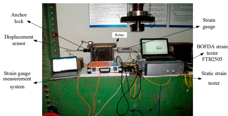
Figure 5. Test system of concrete drawing experiment.
