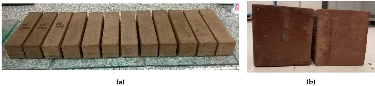
**Figure 6.** Specimen for determination of hardened properties; (a) prisms 40 mm × 40 mm × 160 mm; (b) samples 100 mm × 100 mm × 50 mm.
