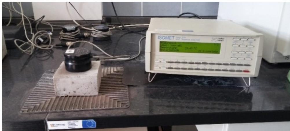
**Figure 14.** Thermal conductivity coefficient determined in a non-stationary method.
