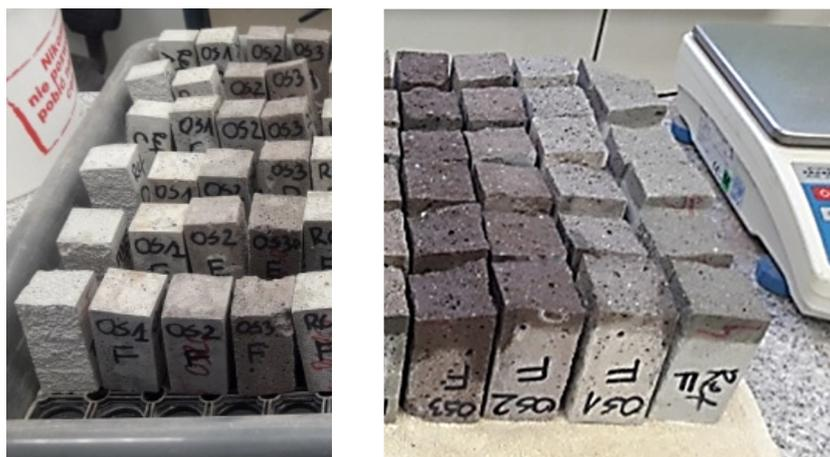
**Figure 15.** Specimen during the determination of water absorption coefficient due to capillary action.
