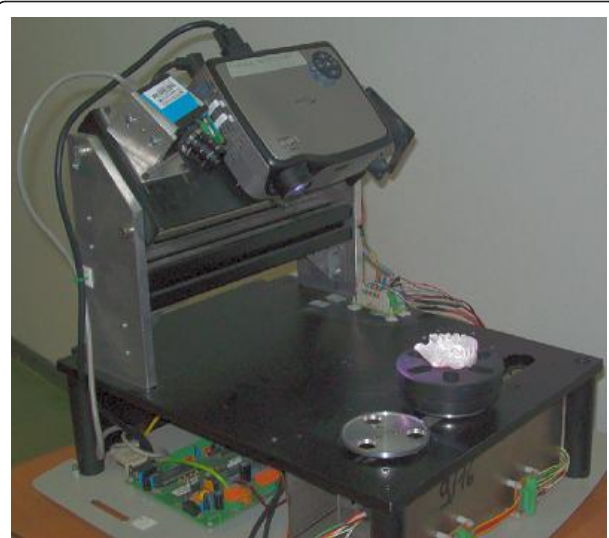
Figure 1 Optical scanner. 3D optical scanner used to capture dental models.
