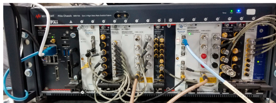
Figure 3. PXIe 8-channel microwave digital receiver.
