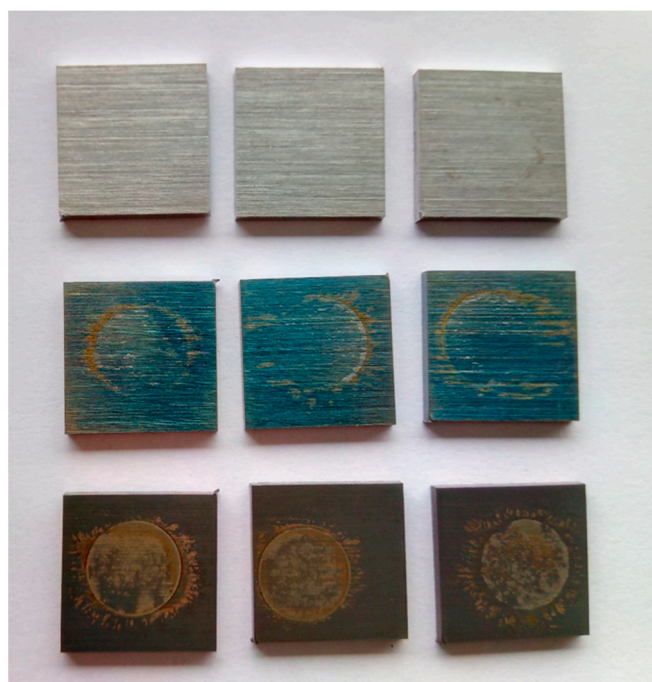
Figure 8. Several 20 mm × 20 mm × 2 mm samples after corrosion analysis, top-bottom; untreated, Plasma 1—CrO, Plasma 2—FeO.
