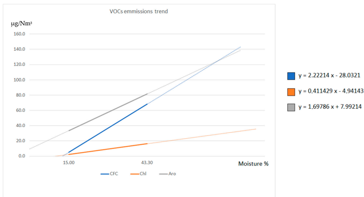
Figure 5. The ideal linear trend in the increase in the concentrations of the VOC classes as a function of the increasing moisture content.
