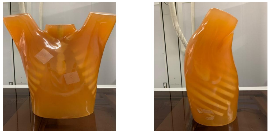
Figure 2. An anthropomorphic chest phantom used in this study.
