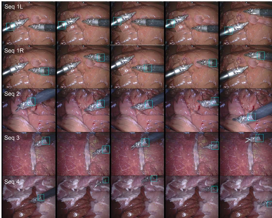
Fig. 13. Result example frames from each sequence of the EndoVis articulated robotic surgical instrument dataset. The result bounding box and centre point is represented in cyan colour, and the ground truth centre point is represented in green colour. (For interpretation of the references to colour in this figure legend, the reader is referred to the web version of this article.)
