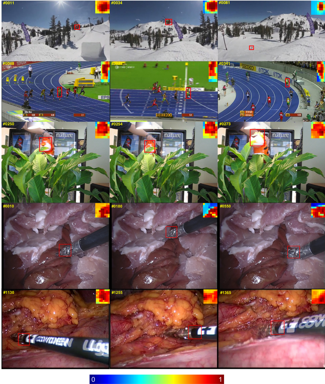
Fig. 3. Example patch weights are shown for the highlighted bounding box displayed in the top corner of the image. Warmer colour indicates higher foreground possibility.
