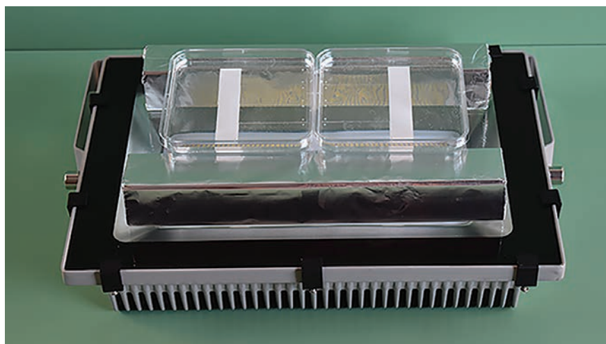
Figure 1. Photobleaching apparatus. The spotlight was placed so that the LED panel was facing upwards and that reflective spacers could be placed on the spotlight protective glass. Above the spacers, two 12-cm square Petri dishes, filled with TRIS buffer added with 0.05% sodium azide, were placed. In the image, the covering glass mirror is not visible.
