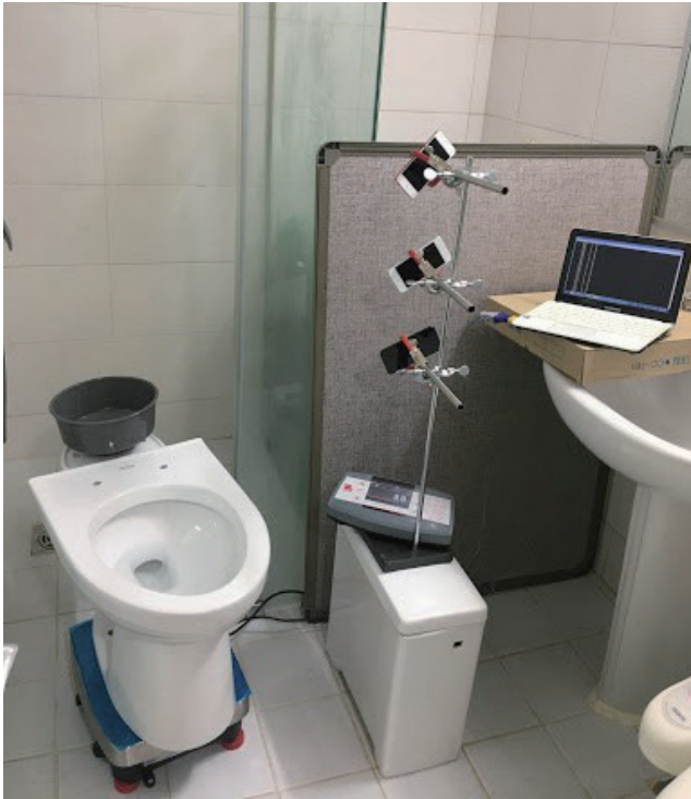
Fig. 2. A laboratory setting to measure the urinary flow while recording urination sound.
