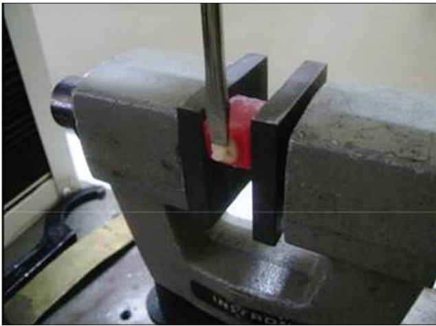
Figure 7: Specimens subjected to shear bond strength evaluation using the universal testing machine
