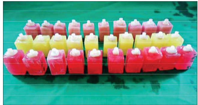
Figure 4: Completed specimens for the evaluation of shear bond strength
