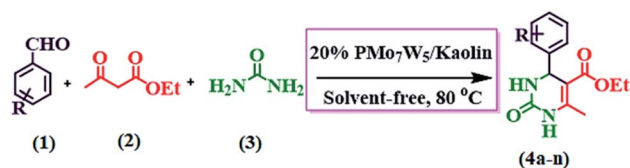
Scheme 3 Synthesis of ethyl 6-methyl-2-oxo-4-aryl-1,2,3,4-tetrahydropyrimidine-5-carboxylate ( 4a-n ) by using 20% \text{PMo}_7\text{W}_5/\text{kaolin} catalyst.
