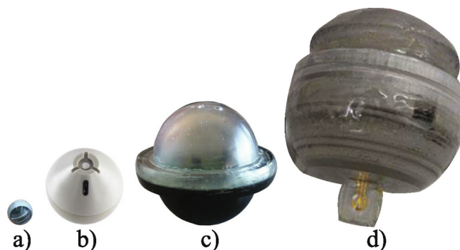
Fig. 3. Instrumented sensor devices: a) Sens-o-sphere [58]. b) smartCAPS (pH version) [42]. c) Bio-capsule [43]. d) bPod [44].
