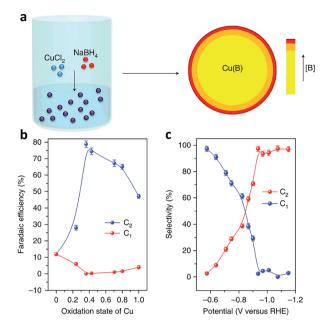
Fig. 14 (a) Schematic illustration of the synthesis of B-doped Cu by a wet-chemical process. (b) Faradaic efficiency of  $C_2$  and  $C_1$  products *versus* the oxidation state of Cu. (c) Selectivity for  $C_2$  and  $C_1$  products at different potentials on B-doped Cu. Reprinted from ref. 93 with permission from Nature Publishing Group.
