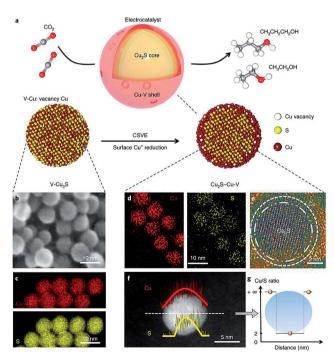
Fig. 15 (a) Schematic illustration of  $Cu_2S-Cu-V$  electrocatalyst design for  $CO_2$  electroreduction to produce multi-carbon alcohols. (b) TEM and (c) EDS mapping of original V-Cu\_2S nanoparticles; (d) EDS mapping, (e) high-resolution TEM, (f) EDS line scan and (g) the ratio of Cu/S concentration of the reduced  $Cu_2S-Cu-V$  electrocatalyst after electrochemical reduction. Reprinted from ref. 61 with permission from Nature Publishing Group.
