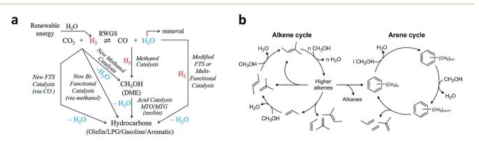
Fig. 7 (a) Schematic illustration of  $CO_2$  hydrogenation to  $C_{2+}$  products *via* the CO intermediate route and CH<sub>3</sub>OH intermediate route. Reprinted from ref. 12 with permission from the Royal Society of Chemistry. (b) General scheme of the dual-cycle mechanism during the MTH process. Reprinted from ref. 44 with permission from Elsevier.
