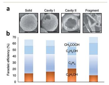
Fig. 13 (a) SEM images of Cu-based catalysts with a morphology of solid, cavity I, cavity II and fragment. Scale bars, 100 nm. (b) Faradaic efficiency of  $C_2$  and  $C_3$  products during CO electroreduction over Cu-based catalysts with the four types of morphologies at an applied potential of -0.56 V *versus* RHE. Reprinted from ref. 89 with permission from Nature Publishing Group.
