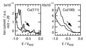
**Fig. 10** Detection of ethylene on Cu (111) (left) and Cu (100) (right) during CO electroreduction by OLEMS. Reprinted from ref. 81 with permission from American Chemical Society.
