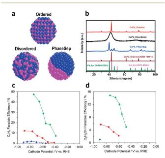
**Fig. 12** (a) Schematic illustration of CuPd nanoalloys with ordered, disordered and phase-separated structures. (b) XRD patterns of the prepared CuPd nanoalloys. Faradaic efficiencies of (c)  $C_2H_4$  and (d)  $C_2H_5OH$  for bimetallic Cu–Pd catalysts with different mixing patterns: ordered, blue; disordered, red; phase-separated, green. Reprinted from ref. 87 with permission from American Chemical Society.
