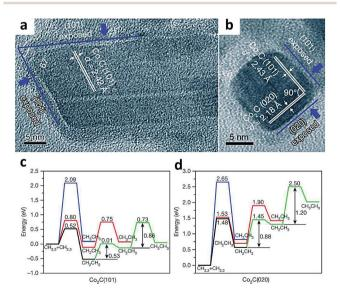
Fig. 2 (a, b) High-resolution TEM images of  $Co_2C$  nanoprisms. Energy profiles for pathways that lead to the formation of  $CH_2CH_2$  and  $CH_3CH_3$  on the (c)  $Co_2C(101)$  surface and (d)  $Co_2C(020)$  surface. Reprinted from ref. 23 with permission from Nature Publishing Group.
