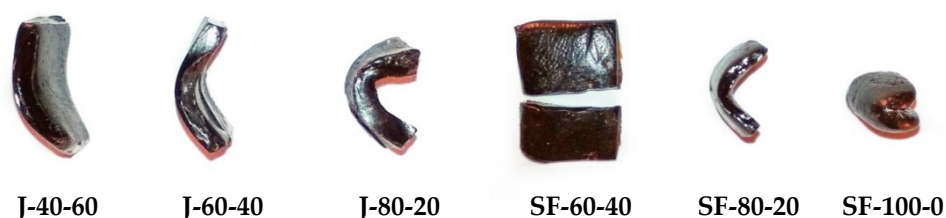
Figure 7. Polymers synthesized with different bismaleimide composition. The codes J and SF refer jatropa or sunflower oil, the numbers describe the percentage of aliphatic and aromatic bismaleimides respectively.
