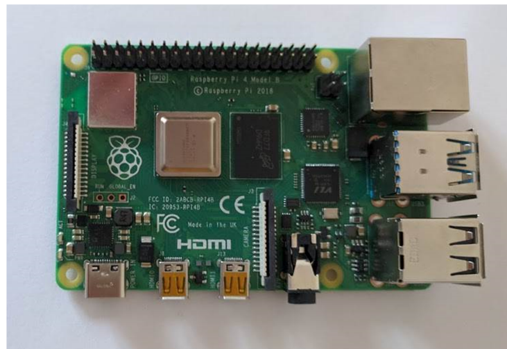
Figure 7. The Raspberry Pi 4 Model B single-board computer used in the proposed framework.
