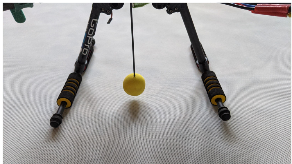
Figure 18. Spherical marker hung under the air station.
