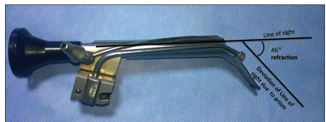
Figure 2: Truview PCD video laryngoscope blade. The 46 degree angle of refraction produced by the prism enables visualization of anteriorly placed structures
