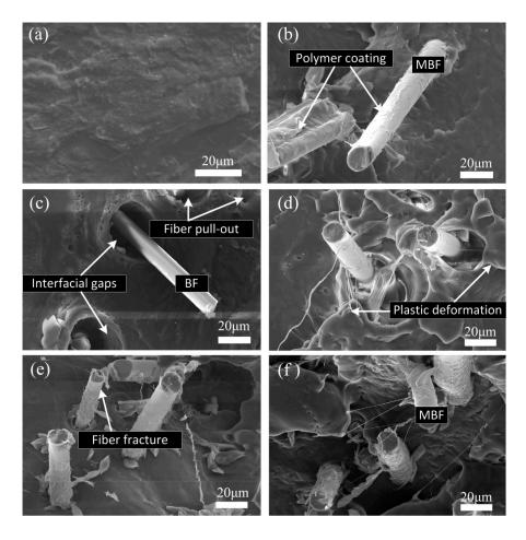
**Figure 9.** Scanning electron microscopy (SEM) micrographs of tensile fractured surfaces of (**a**) PBS, (**b**) PBS/MBF (98/2), (**c**) PBS/BF (95/5), (**d**) PBS/MBF (95/5), (**e**) PBS/MBF (90/10), and (**f**) PBS/MBF (85/15).
