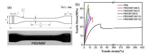
Figure 8. (a) Standard tensile samples; (b) stress-strain curve of PBS, PBS/BF, and PBS/MBF.
