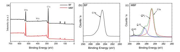
**Figure 2.** (a) X-ray photoelectron spectrometer (XPS) wide scan spectra of basalt fiber (BF) and modified basalt fiber (MBF) with labeled photoelectron (C1s, O1s, and N1s), and XPS high resolutions, C1s spectra of (b) BF and (c) MBF.
