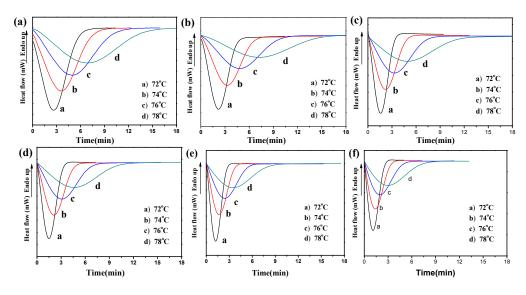
**Figure 5.** Differential scanning calorimetry (DSC) thermograms of (**a**) PBS, (**b**) PBS/MBF (98/2), (**c**) PBS/BF (95/5), (**d**) PBS/MBF (95/5), (**e**) PBS/MBF (90/10), and (**f**) PBS/MBF (85/15) at different crystallization temperatures.
