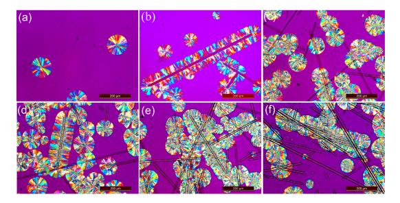
**Figure 3.** Polarized optical microscope (POM) images of (**a**) PBS, (**b**) PBS/MBF (98/2), (**c**) PBS/BF (95/5), (**d**) PBS/MBF (95/5), (**e**) PBS/MBF (90/10), and (**f**) PBS/MBF (85/15) at 89 °C for 35 min.
