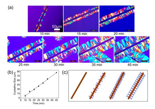
**Figure 4.** (a) The growth of transcrystallization (TC) on MBF of PBS/MBF (98/2) composites crystallized at 89 °C with different time; (b) thickness of TC layer; (c) schematic illustration of TC structure.
