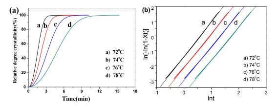
**Figure 6.** (a) Relative degree of crystallinity with time and (b) the Avrami plots of  $\ln[-\ln(1 - X_t)]$  versus  $\ln t$  for isothermal crystallization of PBS/MBF (95/5) at different crystallized temperatures.
