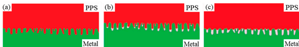
Figure 10. Schematic representation of three filling models. (a) completely filled; (b) partially filled; (c) unfilled.
