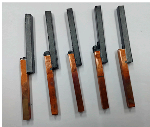
Figure 8. Schematic representation of the copper-PPS assemblies.
