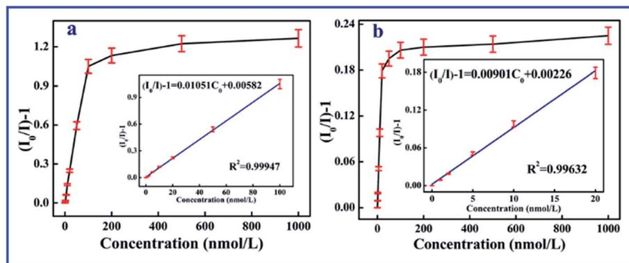
Fig. 2 Linear response of the SiO<sub>2</sub>@dye-MIPs (a) and SiO<sub>2</sub>@dye-NIPs (b) to 2,4,6-TCP in the concentration range from 0 to 1000 nM.
