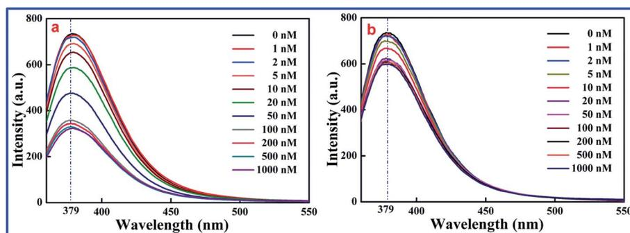
Fig. 1 Response of SiO<sub>2</sub>@dye-FMIPs (a) and SiO<sub>2</sub>@dye-FNIPs (b) to 2,4,6-TCP in the concentration range from 0 to 1000.0 nM.
