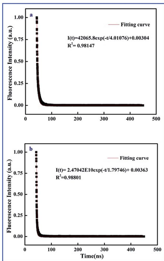
Fig. 3 Time-resolved fluorescence curves of SiO<sub>2</sub>@dye-FMIPs before (a) and after (b) adsorbing 2,4,6-TCP.
