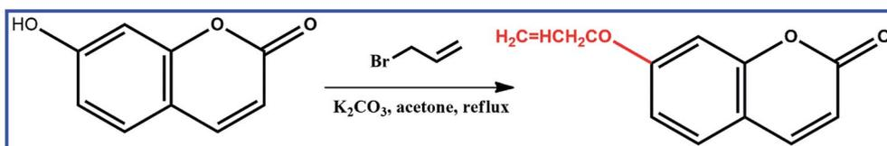
Scheme 1 Schematic illustration of the synthesis of 7-allyloxycoumarin.
