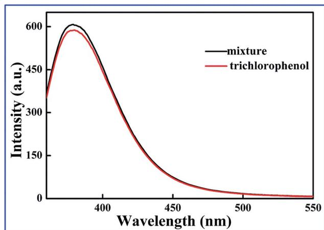
Fig. 5 Test for the interference of different chlorophenols on the fluorescence response toward 2,4,6-TCP of SiO<sub>2</sub>@dye-FMIPs sensor.
