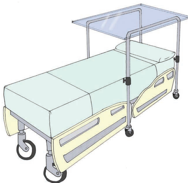
Figure 2. A possible easy-to-arrange bedside barrier between patients and operators for highly contagious aerosolized respiratory fluids.
