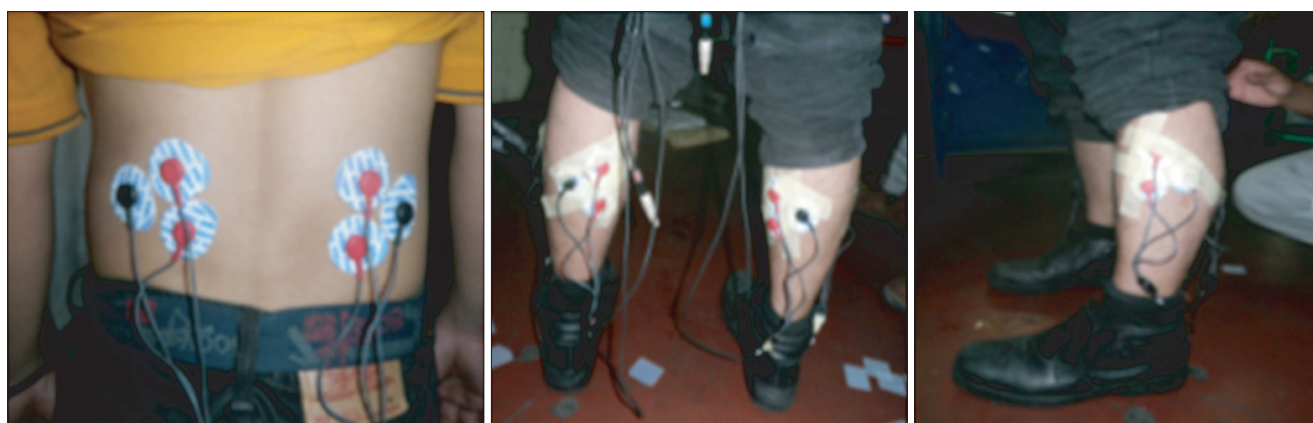
Fig. 2. Surface electrodes (Ag/AgCl) are attached over the erector spinae muscles (lower back), gastrocnemius muscles (posterior legs) and tibialis anterior muscles (anterior legs).
