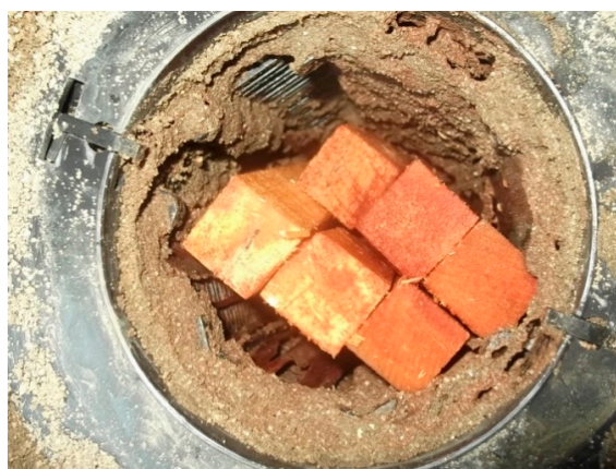
Figure 2. Wooden stakes were placed inside inground monitoring station (IGS).
