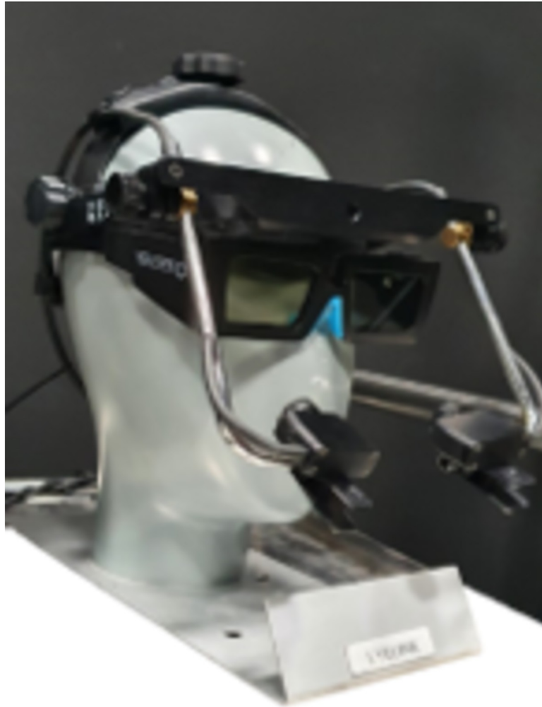
Fig 2. Eye tracker and occlusion glasses worn by the participant.
