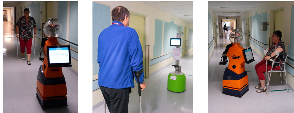
Figure 1. Patients during SAR-based self-training, where training robots drive in front of the patients and provide motivational and corrective feedback on their gait behavior ( left, middle ). Patients can pause the training at resting places ( right ).
