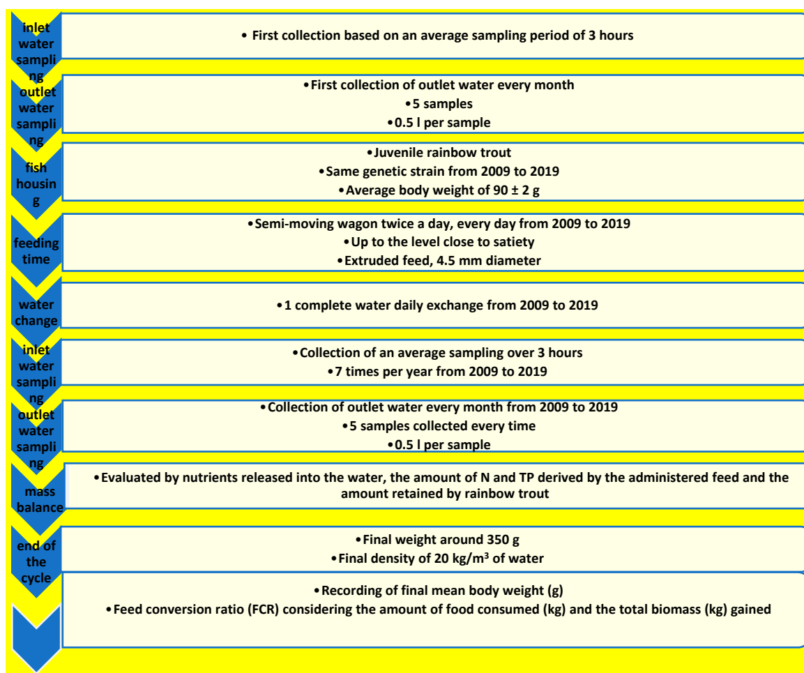
Figure 1. Diagram showing the experimental design adopted during the 10 years of the study.
