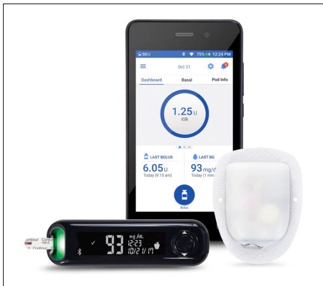
Figure 1. Omnipod DASH™ Insulin Management System Personal Diabetes Manager (PDM) and Pod, with the interoperable CONTOUR® NEXT ONE blood glucose meter.
