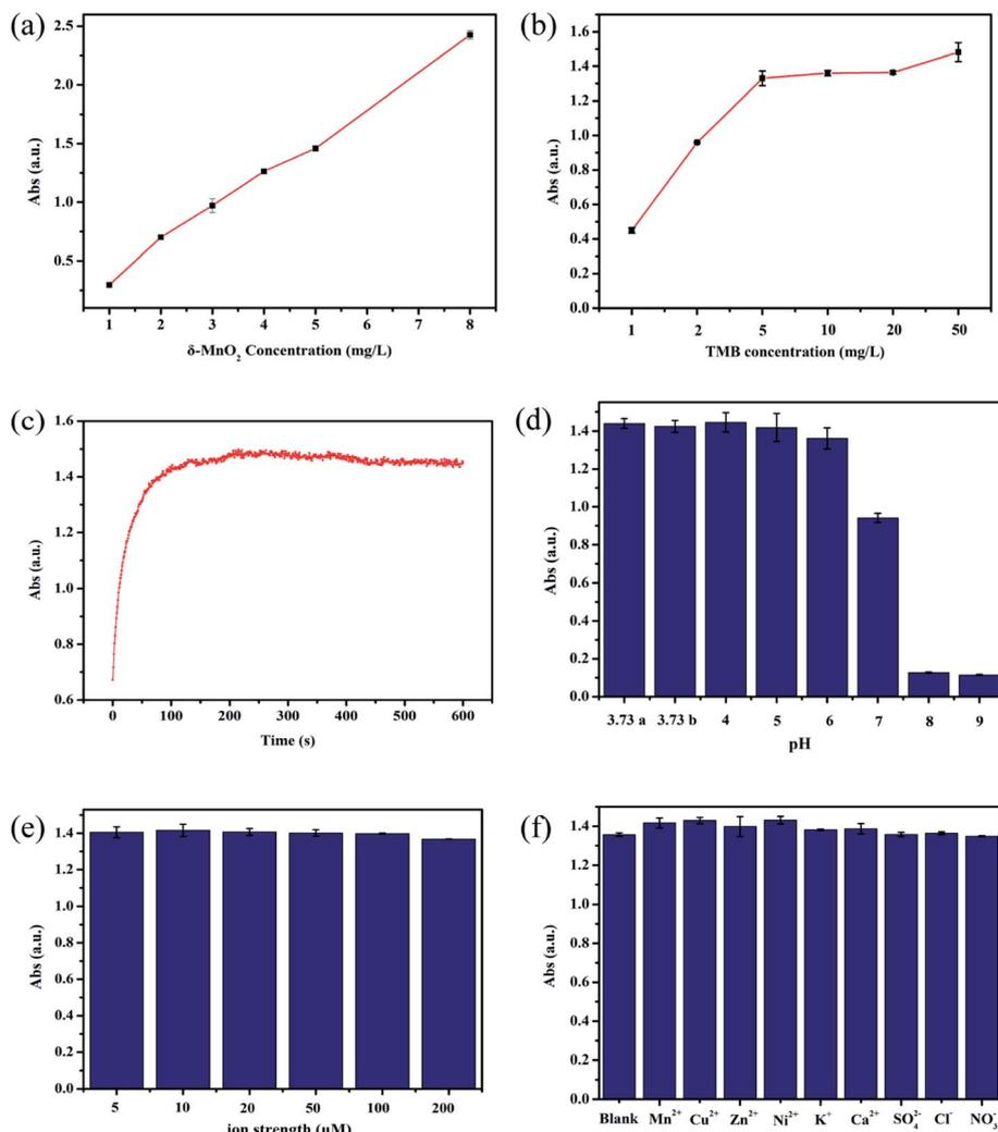
Fig. 1 Effects of a variety of factors on the TMB oxidase-like activity of  $\delta$ -MnO<sub>2</sub>. (a) Effect of  $\delta$ -MnO<sub>2</sub> concentration. (b) Effect of TMB concentration. (c) Effect of reaction time. (d) Effect of pH. 3.72a was assayed in 100 mM NaCl, while 3.72b was assayed in HAC–NaAC buffer. (e) Effect of ion strength. (f) Effect of common anions and cations.
