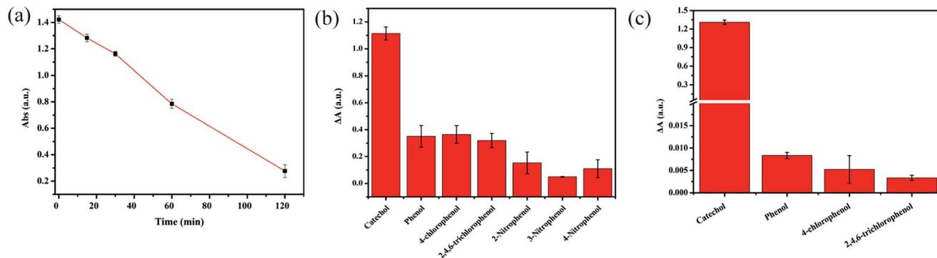
Fig. 3 (a) The effect of incubation time of catechol and  $\delta$ -MnO<sub>2</sub> (b) detection selectivity of  $\delta$ -MnO<sub>2</sub>-TMB to different phenolic compounds at pH 3.73 (c) detection selectivity of  $\delta$ -MnO<sub>2</sub>-TMB to different phenolic compounds at pH 6.00.
