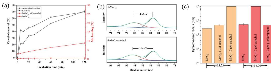
Fig. 4 (a) Catechol removal and Mn(II) leaching profiles during the incubation process. The initial amount of MnO<sub>2</sub> was 50 mg L<sup>-1</sup>, and the catechol was 150  $\mu$ M (b) Mn 3s spectra of the pristine  $\delta$ -MnO<sub>2</sub> and catechol reacted  $\delta$ -MnO<sub>2</sub>. (c) DLS results of pristine  $\delta$ -MnO<sub>2</sub>, and  $\delta$ -MnO<sub>2</sub> treated with catechol and *p*-chlorophenol.
