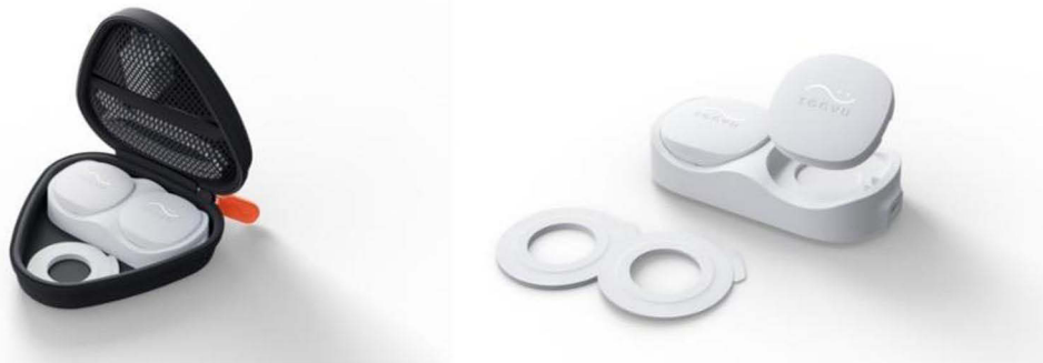
Figure 1 Pictures of the experimental device. Left shows the pods resting in the charging cradle inside the carrying case. Right shows pods, charging cradle, and two adhesive rings.
