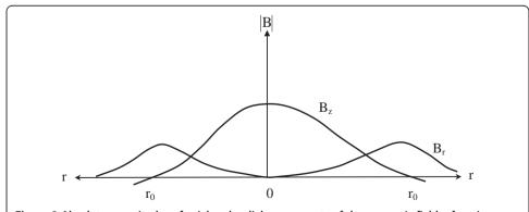
Figure 2 Absolute magnitudes of axial and radial components of the magnetic field a function radial distance from the central z-axis of the coil. Sketched from Alfonsetti et al. 2010 [21], and Cohen et al. 1990 [22].
