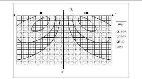
Figure 5 Contour plot of the electric field induced by a neurostimulating coil (solid dots) in a central plane below a one-turn coil of radius R. The coil is parallel the surface (z = 0) of a semi-infinite volume of homogenous tissue. Field vectors are perpendicular to the plane of the page. Contour intervals are 5 V/m apart.
