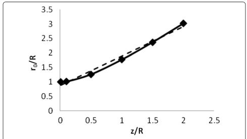
Figure 4 Extent,  $r_0$ , of the dome shaped region of positive z-directed magnetic field as a function of axial depth beneath a simple circular coil. The linear regression function (dashed line) is y = 1.02x + 0.87.
