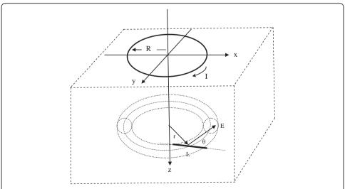
Figure 9 Axon penetrating a torus of induced voltage and current. Heavy line represents the axon segment of length, L, which transects a local field of induced EMF at angle  $\theta$ .
