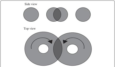
**Figure 15** Joint induced voltage and current fields of figure of eight coils in a semi-infinite uniform volume conductor. A spindle shaped volume of overlapping induced EMF is created.
