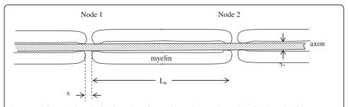
**Figure 8 Schematic longitudinal section of a myelinated axon.** The width of each node of Ranvier is denoted s. The distance between nodes is denoted  $L_n$ . This sketch is foreshortened in the axial dimension. Anatomically  $L_n/s \sim 1000$ .
