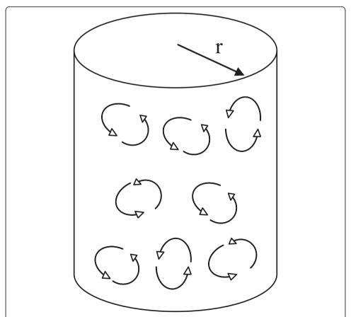
Figure 3 Visualizing EMFs and currents induced by radial components of the B-field beneath a current carrying coil. Induced currents in any potential loop tend to be cancelled by those in neighboring loops.
