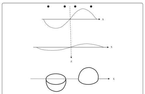
**Figure 13 Joint B-fields of figure of 8 coils (top) and bowl metaphor (bottom).** Figure of eight coils with counter-rotating currents are aligned with the x-axis. B-fields from the two coils and their time derivatives are opposite in sign. As they rise and fall in time counter-rotating eddy currents are induced in underlying tissue which reinforce at points near the z-axis.
