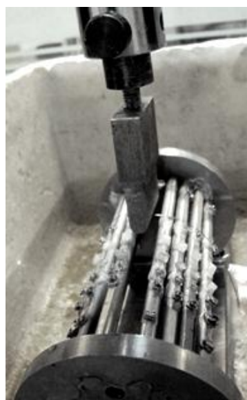
Fig. 4. Three-point bending test of the mounted arch wire kept in a water bath at a constant temperature of 35.5°C
