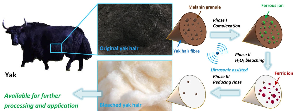
Fig. 1. Proposed ultrasonic-assisted bleaching strategy for yak hair.
