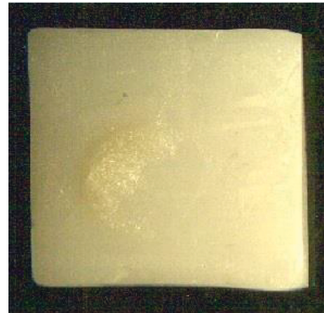
FIGURE 7: Mixed failure mode observed in zirconia-feldspathic ceramic assembly.
