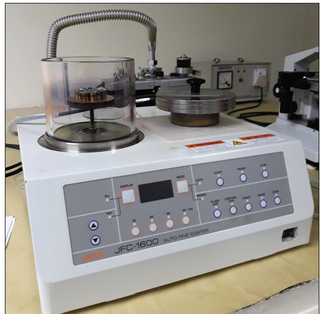
Figure 2: Gold sputter coating of the specimens.
