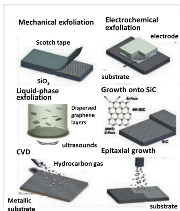
Figure 3. Most typical techniques for graphene synthesis.
