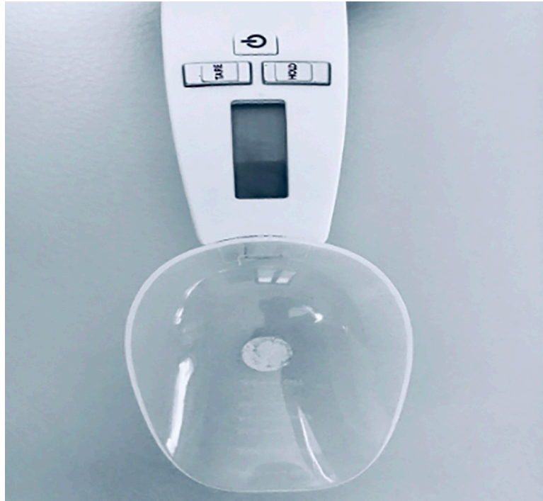
Fig 1. Digital spoon model showing “On/Off” button, “TARE” and “HOLD” buttons and spoon bowl.
