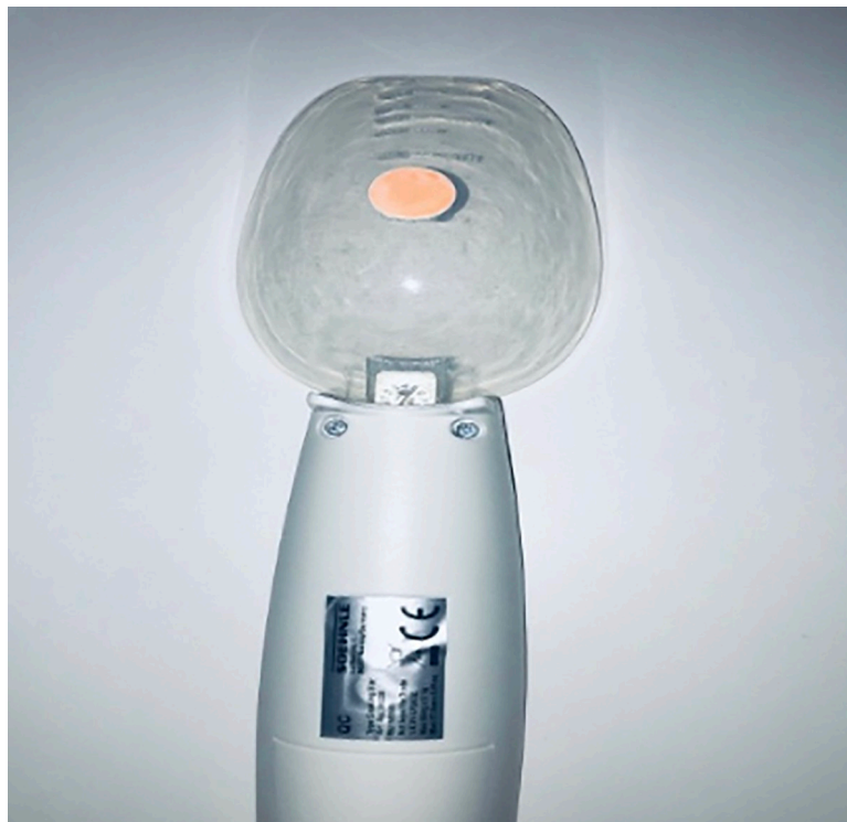
Fig 2. Back of the digital spoon with the 1-cm 2 sticker placed in the middle (point of maximum support) to take measurements.
