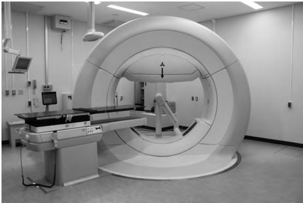
Fig. 1. External appearance of the Vero4DRT installed in Kyoto University. The X-ray head (indicated by an arrow) can rotate 360 degrees along the inner surface of the O-ring. Here, the O-ring gantry is also rotated around the vertical axis, which enables non-coplanar beam delivery without rotating the couch.
