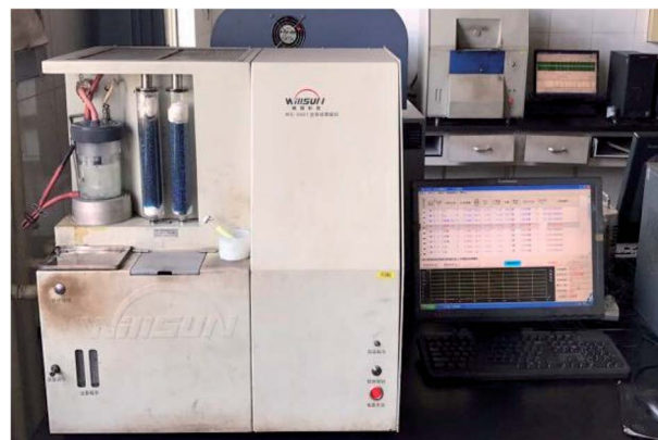
Fig. 4 The automatic sulfur meter (WS-S501).
