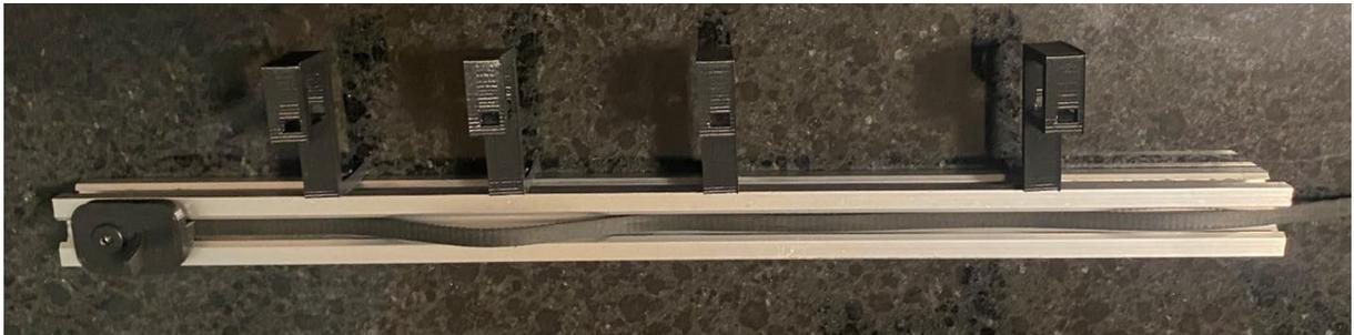
**Fig. 14.** Installation of cable guides, belt, and belt clamp on gantry.
