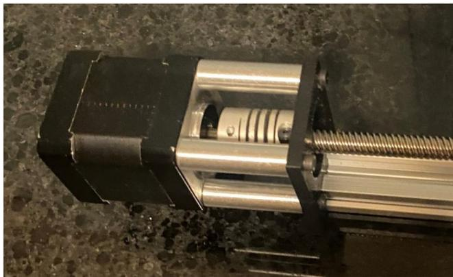
**Fig. 28.** Attachment of Z-axis stepper motor to motor mount with 35 mm spacers.
