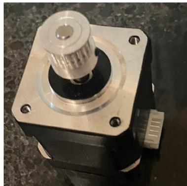
**Fig. 10.** Timing pulley installed on Nema 17 stepper motor.
