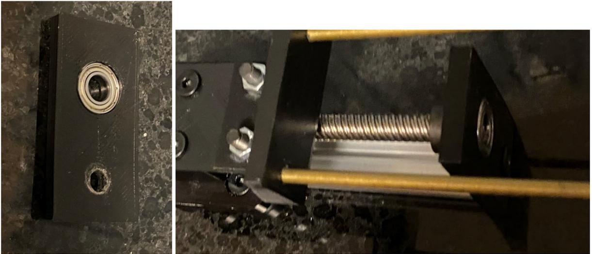
Fig. 25. Assembly and installation of Z-axis end plate.
