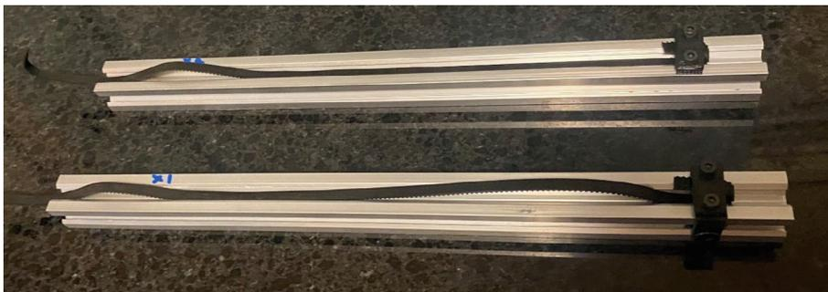
**Fig. 8.** Installing timing belts on x-rails.
