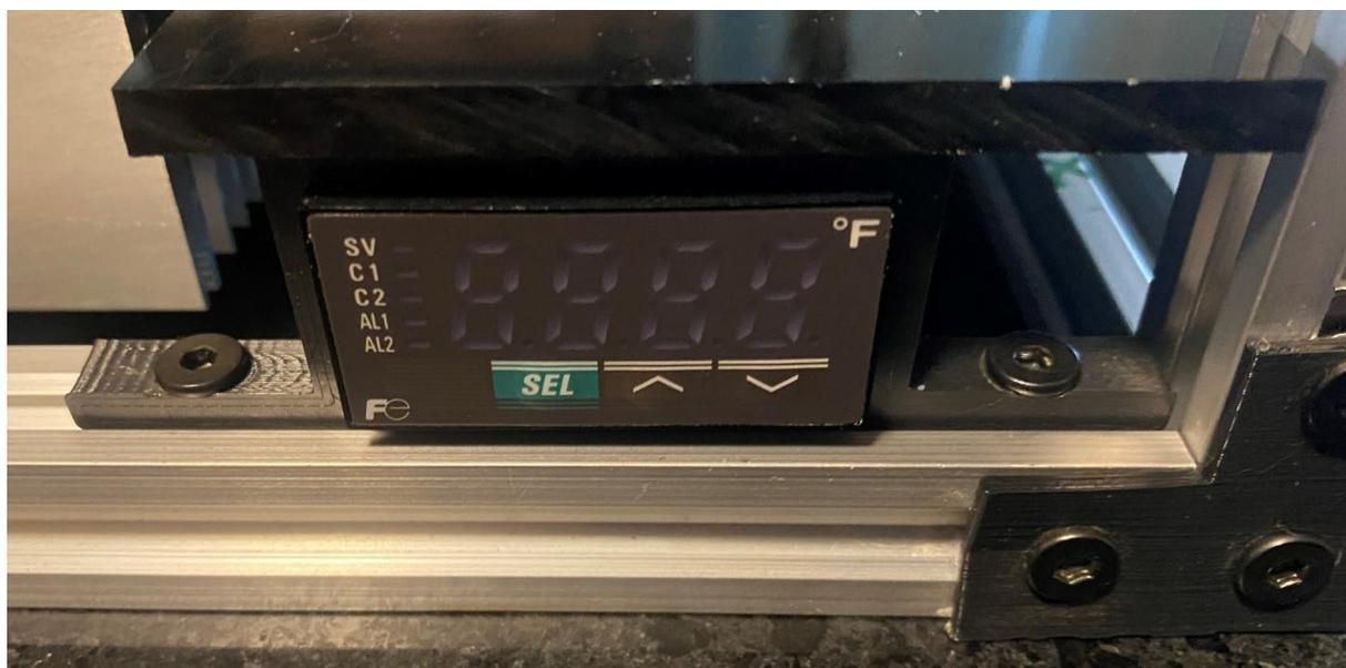
**Fig. 51.** Mounting of temperature controller.
