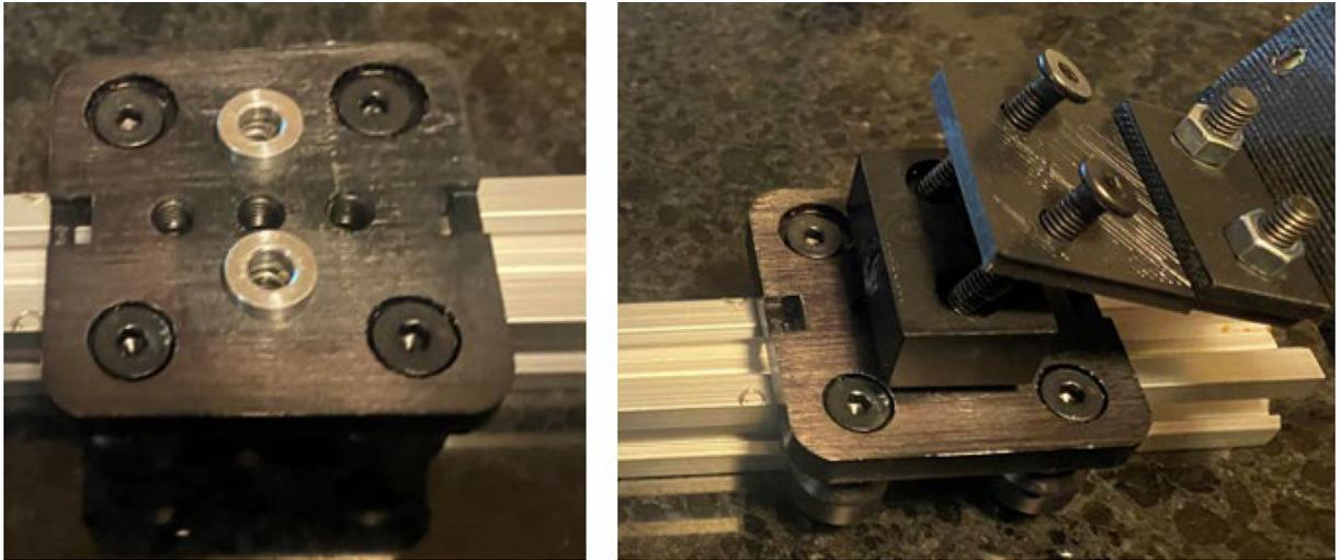
Fig. 22. Attachment of Capillary Holder to Z-axis gantry.
