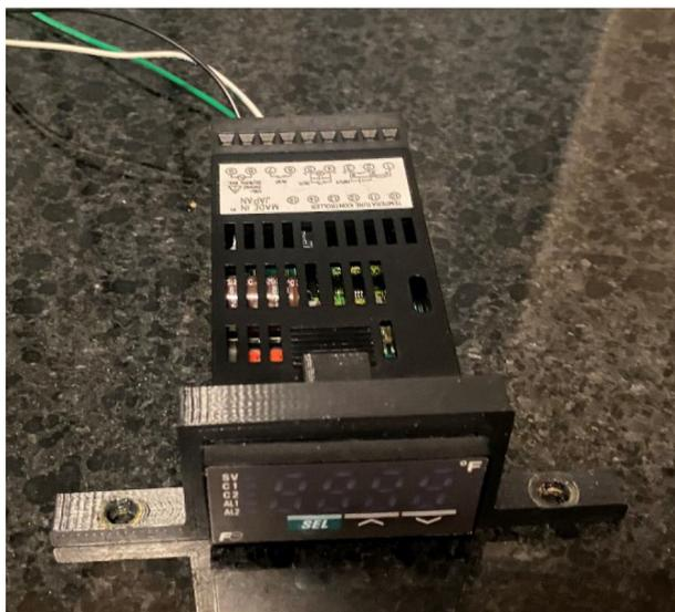
Fig. 35. Temperature controller installed in mount.
