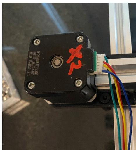
Fig. 61. X2 motor cable connection.
