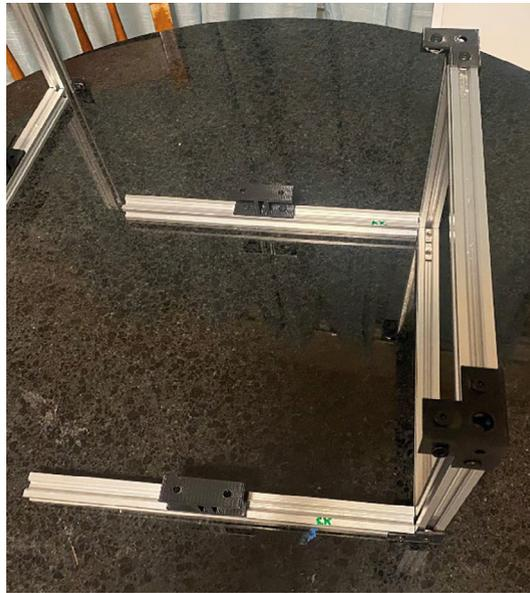
Fig. 5. X rails coupled to front frame.
