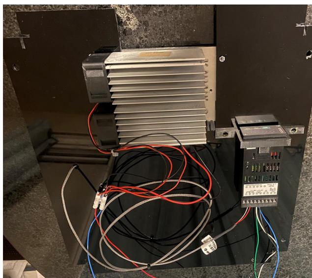
Fig. 36. Underside of acrylic base plate showing position of Peltier chiller assembly and temperature controller connections.
