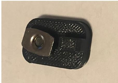
**Fig. 13.** Belt clamp with t-nut installed.
