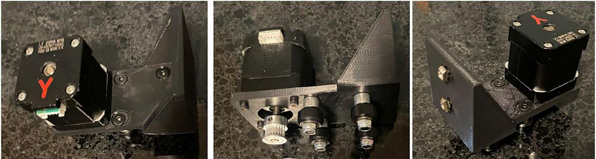
Fig. 11. Installing Y stepper motor and drop-in T-nuts on Y motor mount.
