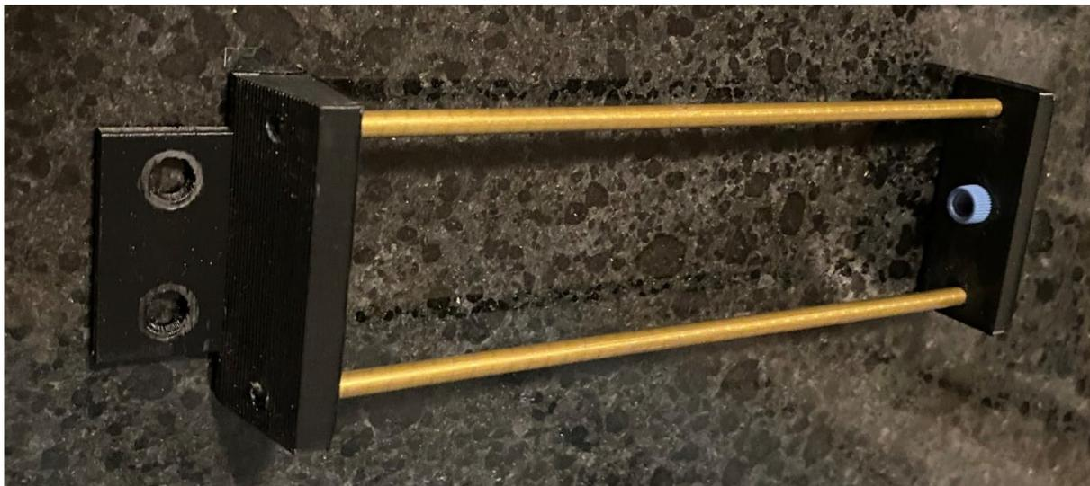
Fig. 18. Assembled capillary holder.
