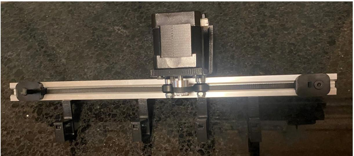
**Fig. 16.** Fixing Y-axis timing belt.
