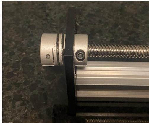
Fig. 26. Installation of shaft coupler.
