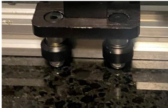
**Fig. 21.** Installation of Z-axis gantry plate.
