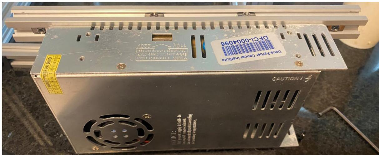
Fig. 48. Power supply coupled to upper Y rail. Note placement of T-nuts for corner connectors.
