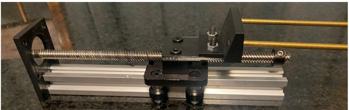
Fig. 24. Threading lead screw into gantry nut block.
