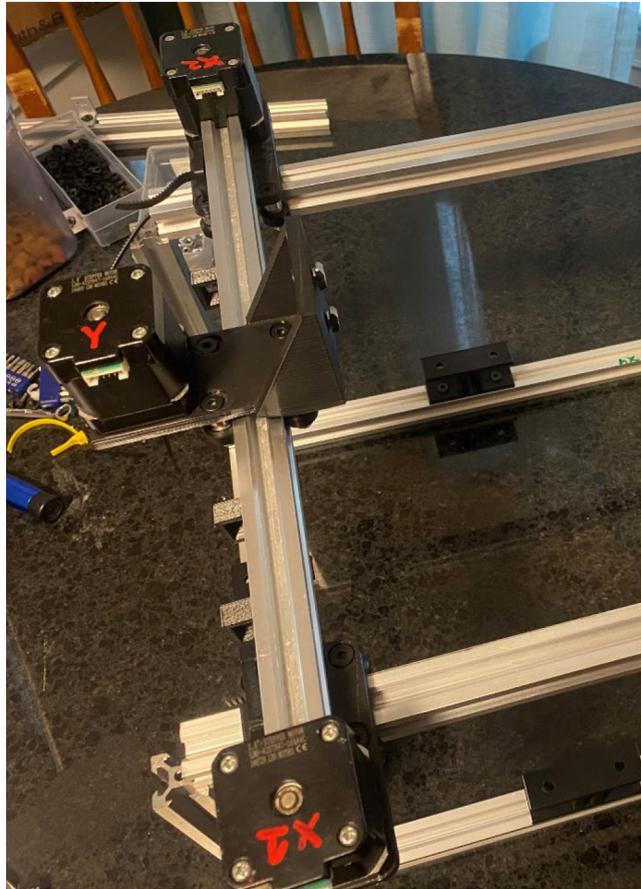
**Fig. 43.** Installing gantry on frame.
