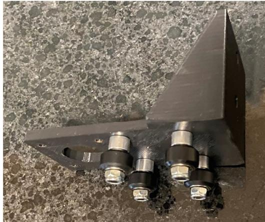
**Fig. 9.** Y motor mount with mini-V wheels installed.
