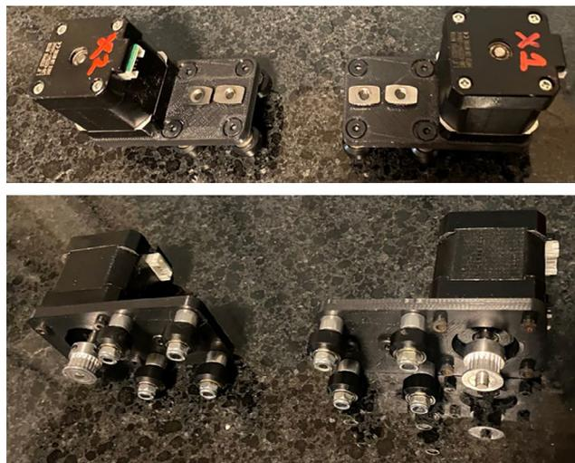
Fig. 12. Assembly of X-axis stepper motors.
