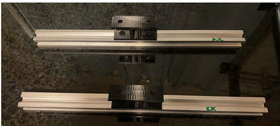
Fig. 4. X-rails with 32 mm spacers.
