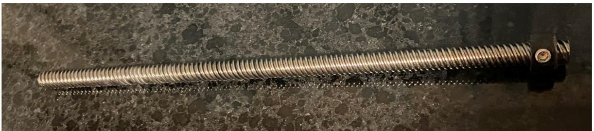
Fig. 23. Install lock collar and shim onto lead screw.
