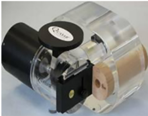
Figure 1 The motion phantom filled with air and a built-in polystyrene cube.
