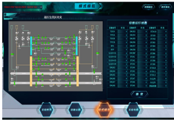
Figure 10. Ventilation control mode design interface.
