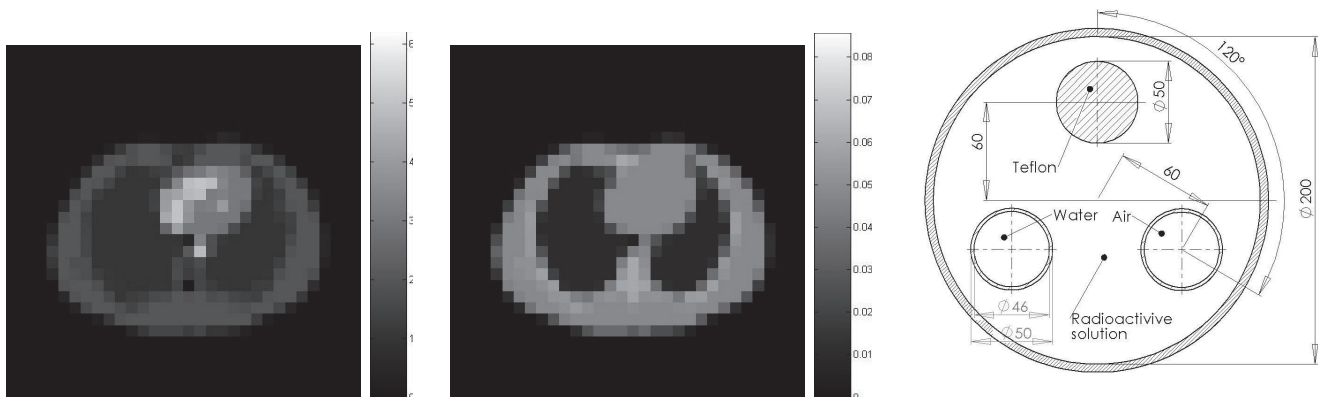
Figure 1. Simulated and physical phantom used in the experiments. From left to right: activity (left) and attenuation (middle) distributions of simulated Zubal phantom, physical imaging phantom with three different material rods inside. (right) doi:10.1371/journal.pone.0106951.g001
