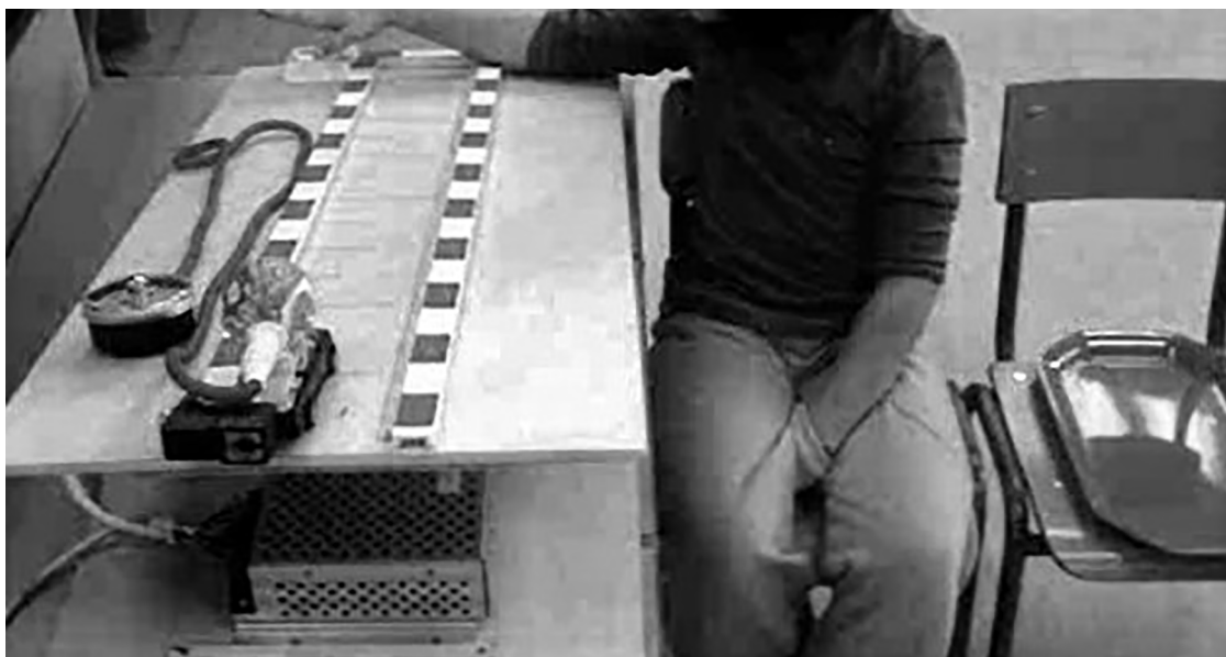
Figure 2. Circuit with different slopes to assess visuomotor coordination, with a car attached to an electromagnet with a dynamometer. Figure shows the child receiving the verbal order “now” and pressing the switch with the affected hand to activate the car. Then, child must transport the car to the tray placed homolateral to the healthy upper limb, thus completing the task, and the total execution time.
