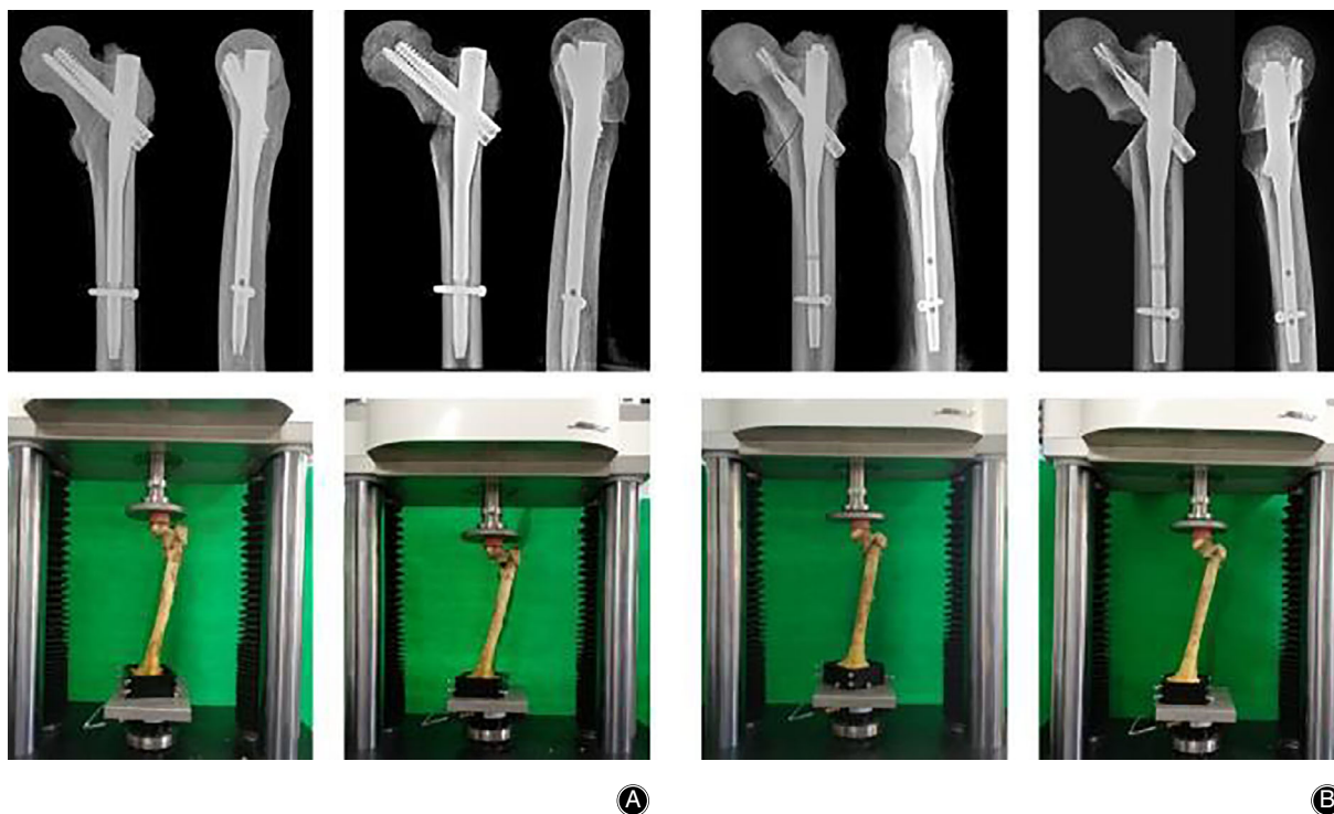
Fig. 2 Radiographs of stable and unstable intertrochanteric fracture with internal fixation and biomechanical loading experiment on Instron testing machine. A-Stable intertrochanteric fracture; B-Unstable intertrochanteric fracture.
