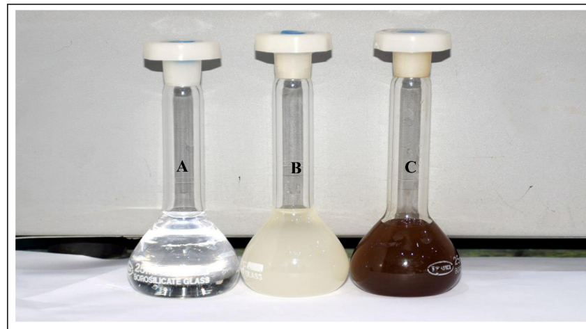
Fig. 5. Culture flasks containing 1-mM \text{AgNO}_3 solution (A), broth containing C. albicans cells (B), and mixture of C. albicans (C) with 1-mM \text{AgNO}_3 .
