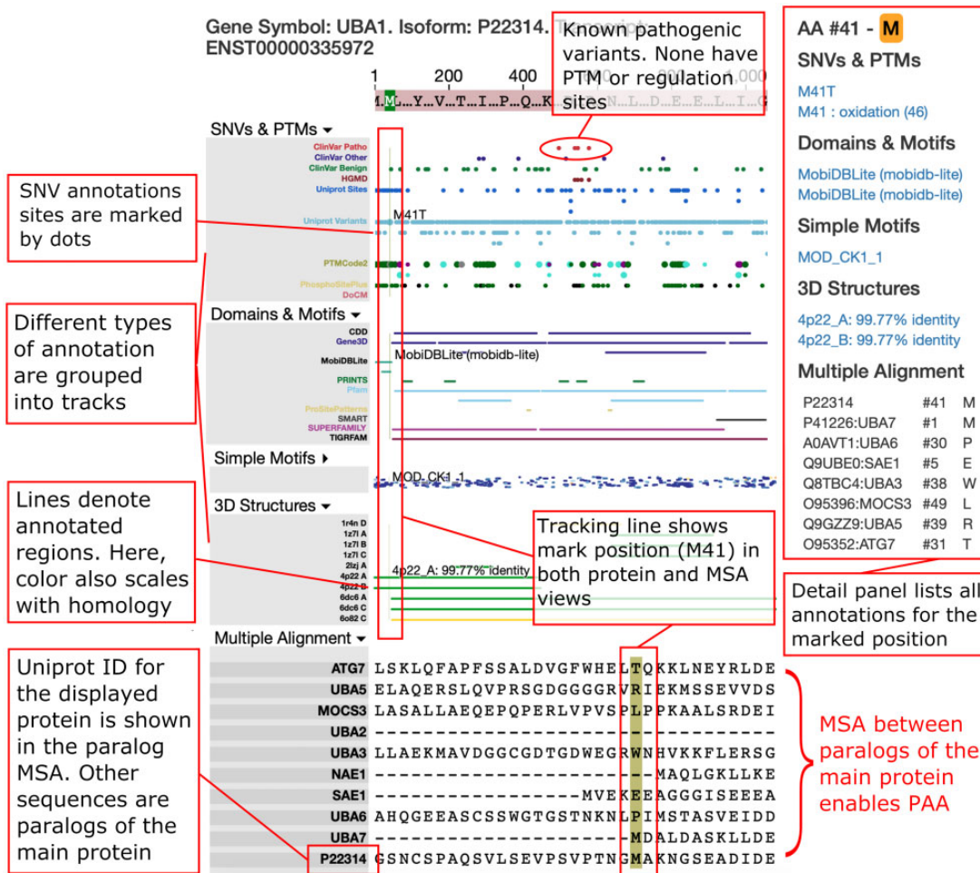
Figure 1. P 2 T 2 for UBA1 demonstrates the rich and comprehensive data that our platform can aggregate and efficiently summarize. When the user places their cursor over an amino acid, the position is highlighted highlight M41 within UBA1, a site with oxidation potential close to the end of an intrinsically disordered region (MobiDB domain is highlighted) and for which homologous experimental structures exist (eg, PDB 4P22 chain A is 99.77% identical). After marking an amino acid, the right-hand panel displays a summary of all available information across that amino acid and the analogous amino acids in the MSA. Color keys for each data type are described in our help page, accessible from the upper toolbar. Pathogenic variants in UBA1 that are associated with muscular dystrophy are noted in the figure. Unlike M41, none of the pathogenic variants are simultaneously annotated with a post-translational regulatory mark.
