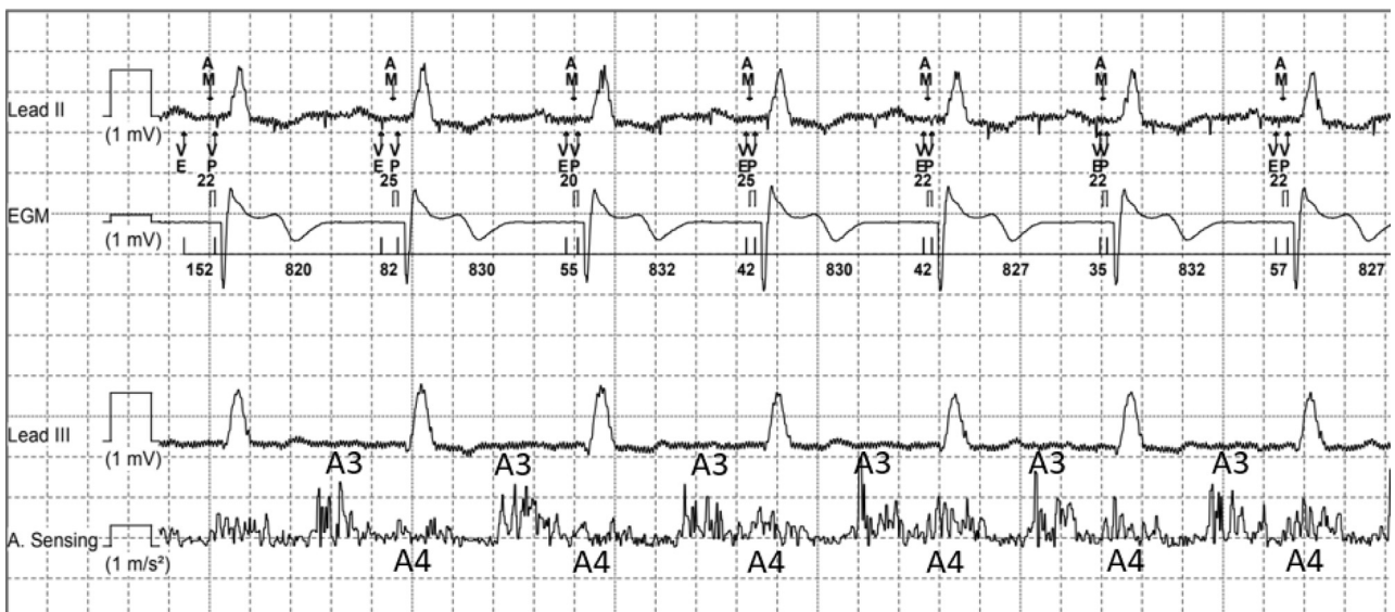
Figure 3 Micra AV (Medtronic, Dublin, Ireland) interrogation postoperative day 1 demonstrates improved sensing of atrial contraction (A4). Marker channels show the timing indicating end of ventricular diastole (A3), labeled as VE (ventricular end). AM (atrial mechanical) is the detection of A4 by the accelerometer, and the delivered right ventricular pacing is VP (ventricular pace).
